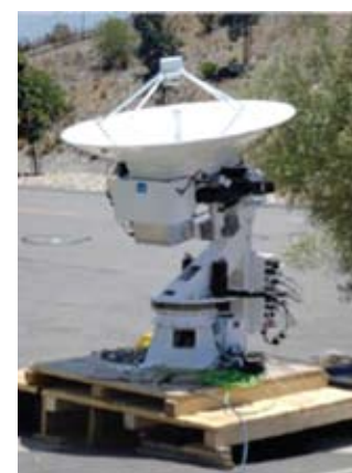
The ePOP ground telemetry station.
