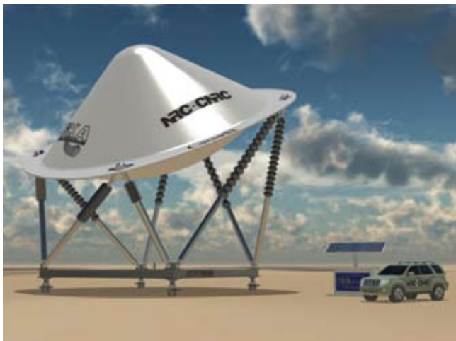
Motive & Klassen original design concept with overconstrained ballscrew drive.
